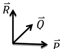
$$(\vec{P} \wedge \vec{Q}) \cdot \vec{R} = \begin{vmatrix} P_X & P_Y & P_Z \\ Q_X & Q_Y & Q_Z \\ R_X & R_Y & R_Z \end{vmatrix} = \text{قيمة سلمية}$$
