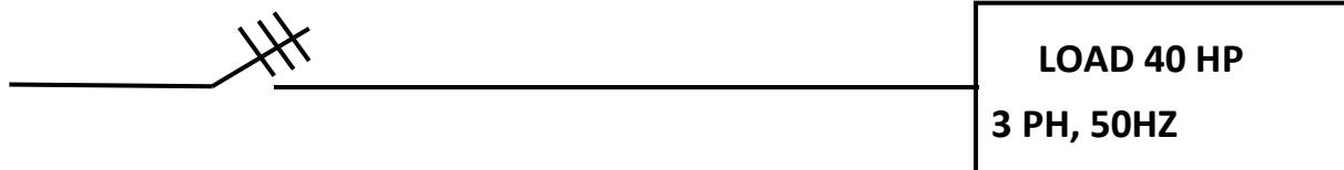
$$I_{rated} = 40 \times 1.5 = 60 \text{ Amp} \quad \text{as } HP = KVA$$
