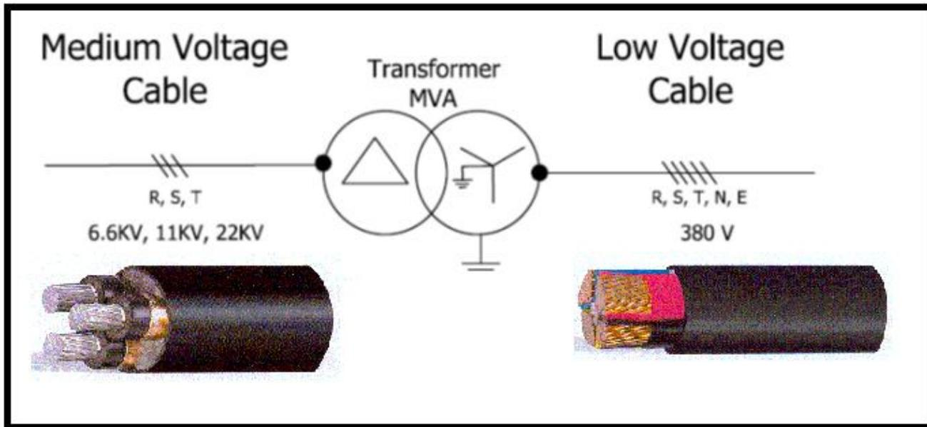
For the same C.S.A medium voltage cable insulation higher than low voltage cables ( $V \alpha$  Insulation).
