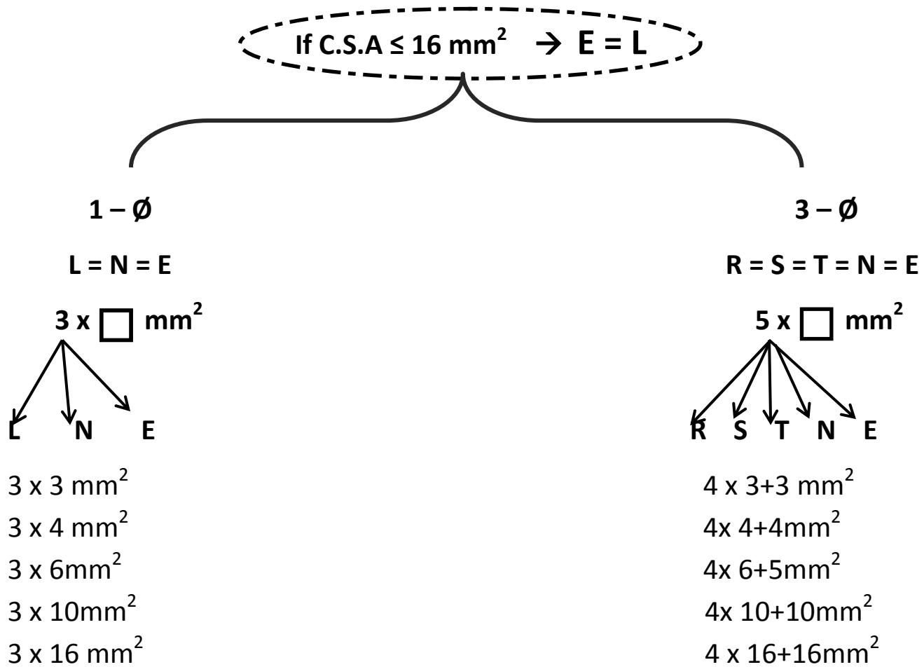
If C.S.A =  $25 \text{ mm}^2$  OR C.S.A =  $35 \text{ mm}^2 \rightarrow E = 16 \text{ mm}^2$
