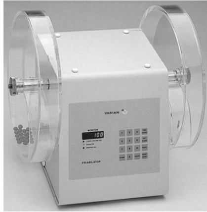
FIGURE 8.14 Varian Friabilator testing apparatus for rolling and impact durability. Tablets are weighed and placed in the acrylic drums, in which a curved baffle is mounted. When the motor is activated by setting the timer, the tablets roll and drop. If the free fall within the drum results in breakage or excessive abrasion of the tablets, they are considered not suited to withstand shipment. The motor makes 20 rpm. When the tablets have been tested, they are removed and weighed again. The difference in weight within a given time indicates the rate of abrasion. (Courtesy of Varian Inc.)
