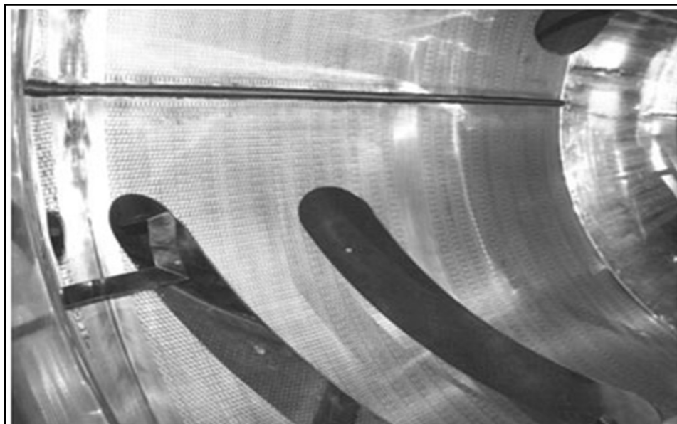
Interior of VHC-66L 1000L Coating Pan Showing mixing baffles, anti-slide baffles, and slotted perforations
